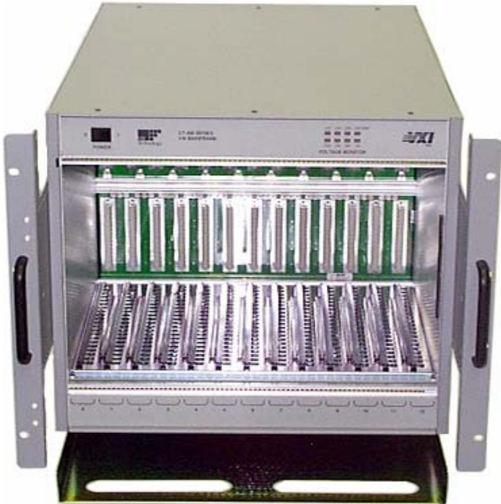
FIGURE 1-6: OPTIONS 100 & 106 - MOUNTING FLANGES/HANDLES & 2U CABLE TRAY
